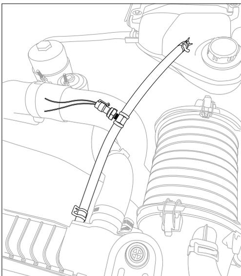
2. Thread the Coolant Pressure Sensor into the selected location and tighten with a 22mm wrench.
