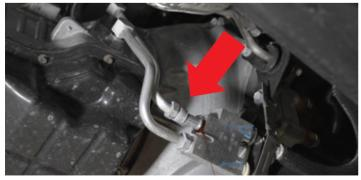
3. Using a Pick Tool, remove the retaining clip and then remove the trans cooler line which leads to the "hot side."
