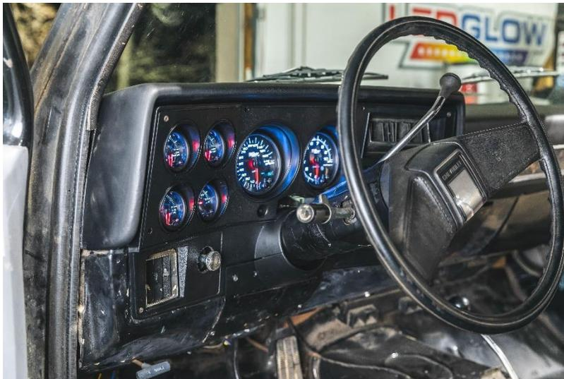
1. Start by removing the screws securing the factory steering column filler panel and cluster trim with a Phillips head screwdriver and remove the factory cluster trim.
