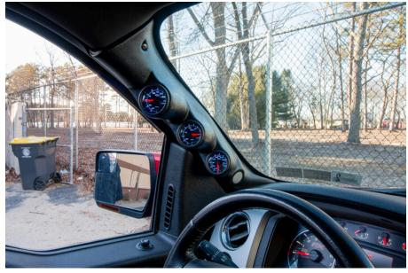
Note: This pillar pod is a complete replacement and will require removal of the factory A-pillar trim. Be sure to store the factory A-pillar trim in a safe location when done.
