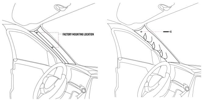
Note: This pillar pod is a complete replacement and will require removal of the factory A-pillar trim. Be sure to store the factory A-pillar trim in a safe location when done.
