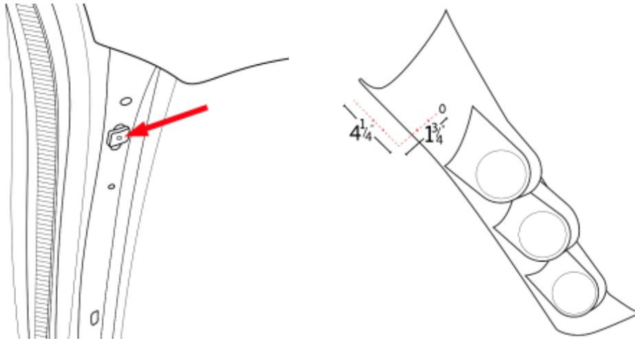
**Note:** This pillar pod is a complete replacement and will require removal of the factory A-pillar trim.
