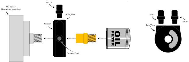
This Oil Cooler Sandwich Adapter is designed for spin on oil filters with a max gasket diameter of 3 inches.
