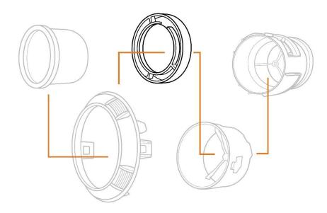
1. Carefully remove the vent assembly by releasing the locking tab at the top of the vent assembly using a small flat screwdriver and turning the inner vent house counterclockwise about and ¼ turn and pulling out.
