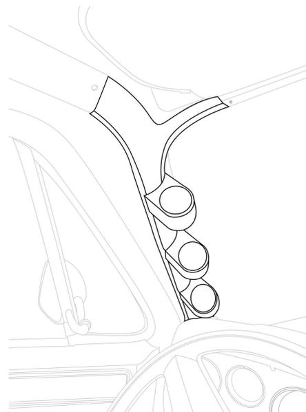
**Note: This pillar pod is a complete replacement and will require removal of the factory A-pillar trim if applicable.**
