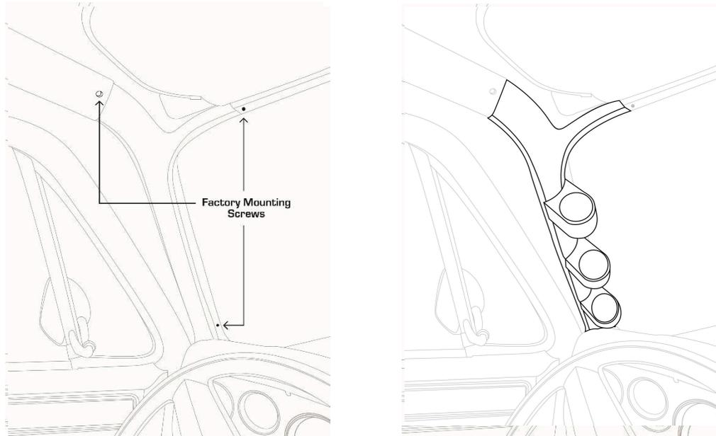
**Note: This pillar pod is a complete replacement and will require removal of the factory A-pillar trim if applicable.**
