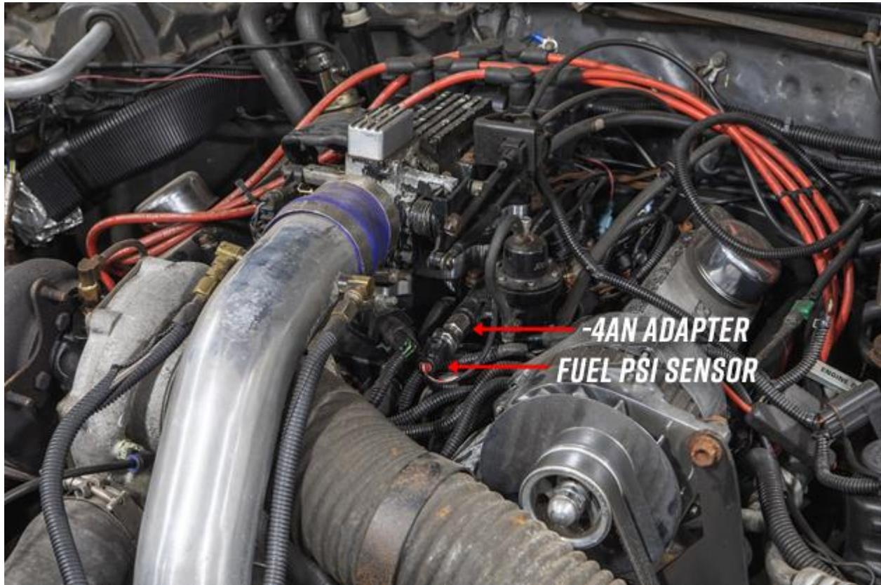
1. Locate the -4AN fuel pressure test port.
