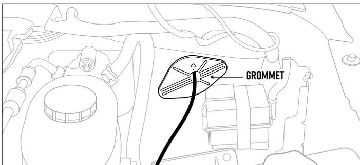
3. Plug the Air Pressure Sensor Harnesses into the Air Pressure Sensors and route through the firewall, keeping them clear of any moving parts and heat sources. Be sure to use a grommet when routing the Air Pressure Sensor Harnesses through the firewall to protect them from being cut or damaged. If one is not available you will need to drill a hole and install a grommet. An extended harness is available on [www.GlowShift.com](http://www.GlowShift.com) if the included harness is not long enough.
