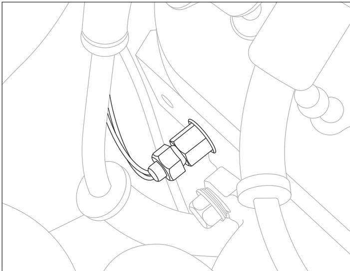
1. There are several different ways to connect a Water Temperature Gauge to your vehicle. In some cases an adapter is needed to adapt the 1/8-27 NPT Sensor.
