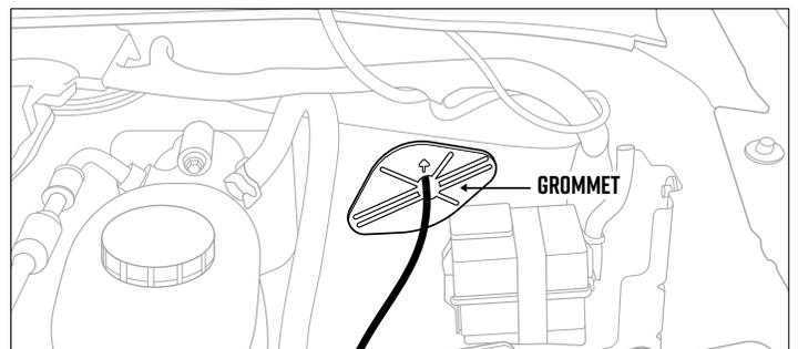
4. Route the **Green Signal Wire** through the engine bay and firewall using a grommet, keeping it clear of any moving parts and heat sources.
