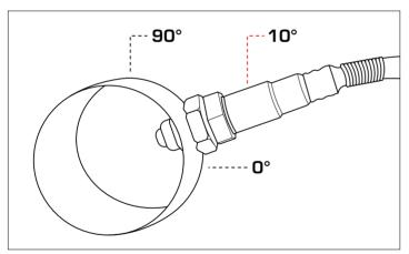
2. To install the weld-in bung, drill a hole into the exhaust using a 15/16" size drill bit. Once drilled, weld the bung to the pipe.
