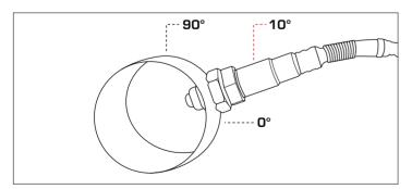
3. To install the weld-in bung, drill a hole into the exhaust using a 15/16" size drill bit. Once drilled, weld the bung to the hole.
