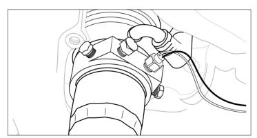
• T-Fitting Installation: Remove your stock oil temperature sensor and fasten a T-fitting in its place. 1/8-27 NPT T-Fittings are available for purchase at www.GlowShift.com. Using a T-fitting allows you to "T" off of the port and open up 3 more, which then allows for the stock and GlowShift sensors to be installed and operate simultaneously. Be sure that Teflon tape is being used on the sensor threads.
